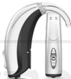
The Widex DREAM power BTE uses our unique wireless WidexLink technology and the new **TRUEISP**, True-Input technology platform. Volume control, program button and telecoil are standard. Uses a size 13 battery.
